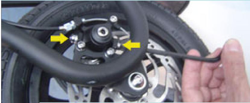
9 The result is the caliper & disc are perfectly aligned ...very important.
